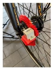
Proper functioning is ensured when the gears of the helical gear interlock in parallel in a line (engagement plane). This can be checked by rotating the front wheel forwards and backwards.
