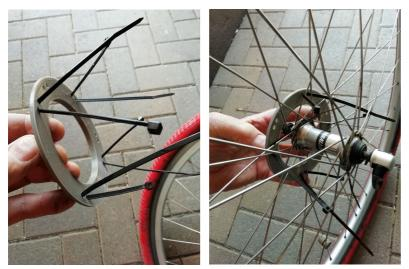
The cable ties are pulled around the crossing point (2 spokes) and closed on the inside (see mounting pictures).
